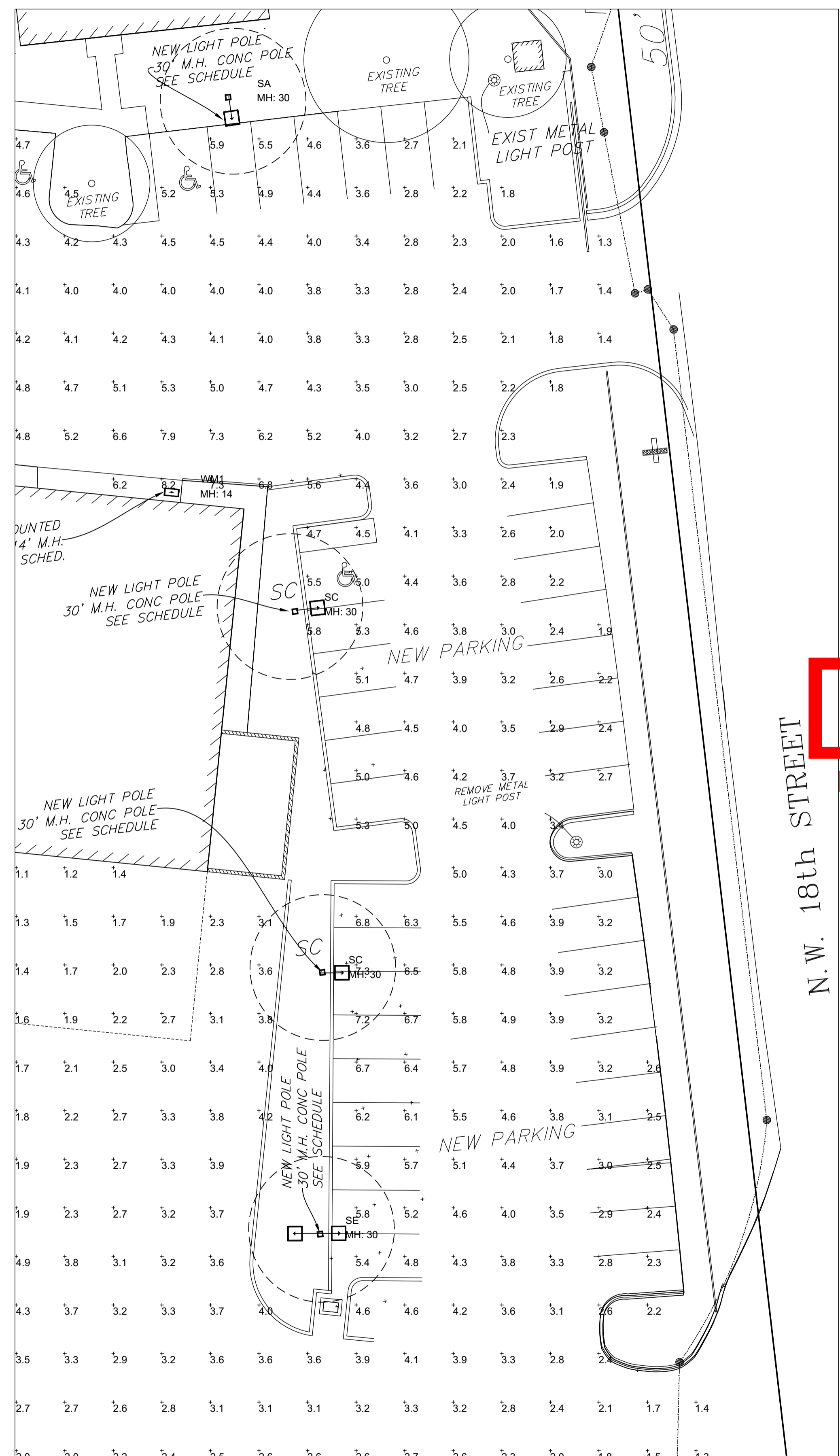
1 PARTIAL SITE LIGHT PHOTOMETRIC PLAN NORTH PARKING SCALE 1/16" = 1'-0"
